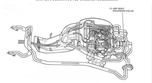
This is the mod for removing the Air Solenoid. What is supposed to happen is the air solenoid which is plugged into the Wiring Harness, is connected to the Speedometer and for speeds below 12Mph the air is taken from the front Ram pipes, for speeds over 12Mph it is taken from the SCOOP. To delete the Air Solenoid, remove the Air Solenoid and front pipes as shown below
