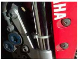
Some people set the front suspension based on rider sag and static sag. This is especially useful in determining if you need softer or stiffer springs. Use the same system as above to determine Rider sag (35-48mm) and Static sag (25-30mm). However I prefer the below method to optimise my current **original** front forks
